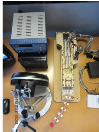
Above: Top View of the Robot. 2 Degrees of freedom (Insertion and Curvature).
