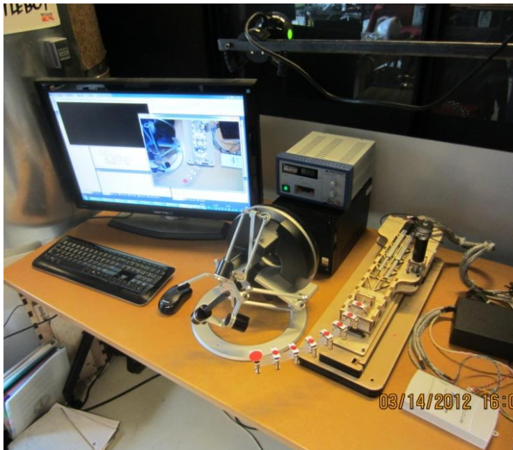
Above: Catheter Robot. Master Controller, Stereoscopic Camera Tracking, Haptic Feedback and Mapping of Environment.
