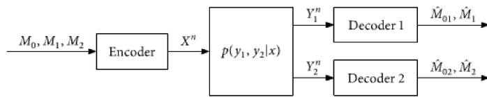
Figure: Two-receiver broadcast communication system [1]
