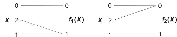
Figure: The deterministic components of the Blackwell channel with state.
