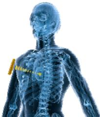
GHz operation frequencies are used to reduce both implant and interrogation system dimensions. Degradation of path loss through tissue at higher frequencies is compensated by higher achievable antenna gain and sensor radar cross sections for fixed size constraints.
